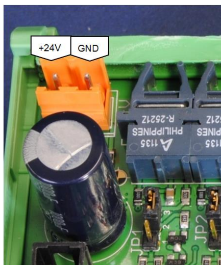
Figure 13: 24 V Voltage supply of the Interlock & Control Module
